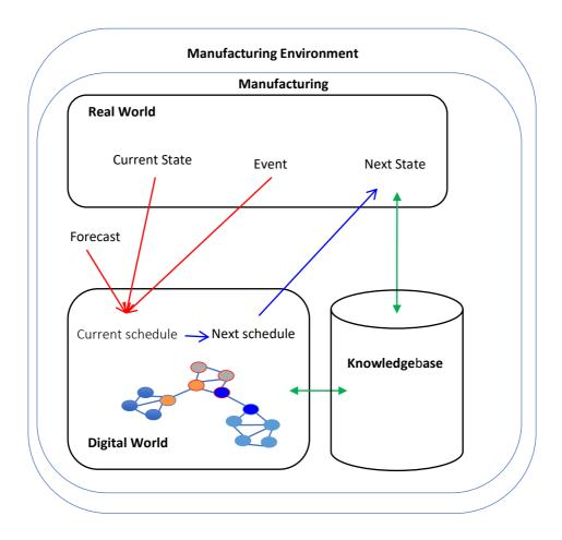
Fig. 1. Architecture of a manufacturing system scheduled by an intelligent real-time scheduler
